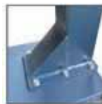
The post will be connected with the chassis with six bolts.
